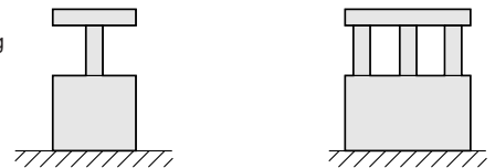
Right angled mounting (2 surfaces and 3 surfaces)
